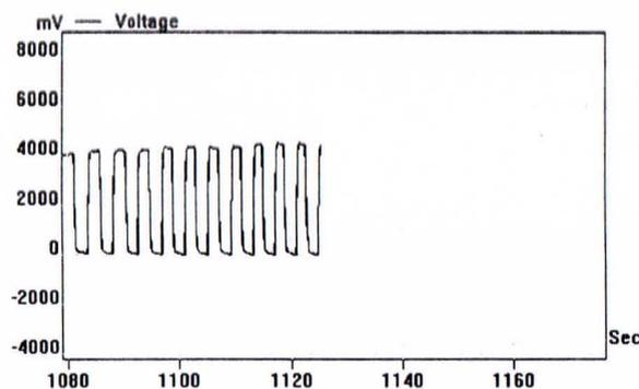
Figure 7. Charge-Discharge measurements for the input current 70 mA with the output voltage 4 Volt.
