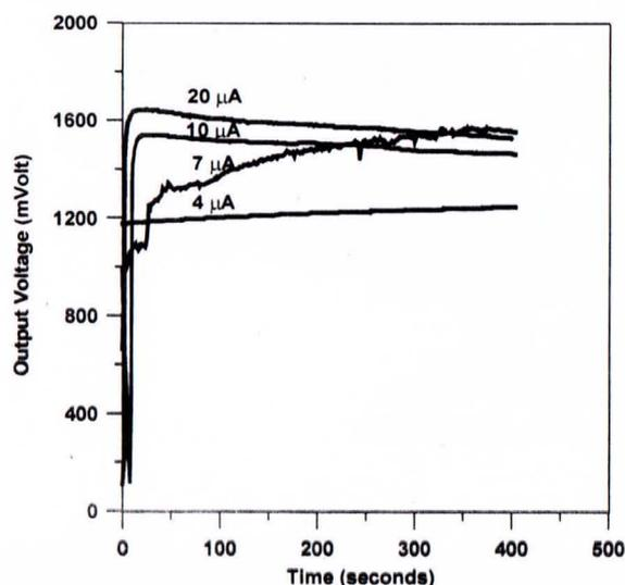
Figure 6. The saturation plot of ionic cell  $\text{Ag}/(\text{AgI})_{0.7}(\text{AgPO}_3)_{0.3}/\text{I}_2$  as a function of given-current.
