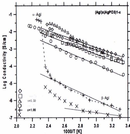
Figure 1. The ionic conductivity of the  $(AgI)_x(AgPO_3)_{1-x}$  as a function of temperature and composition (x) [4].
