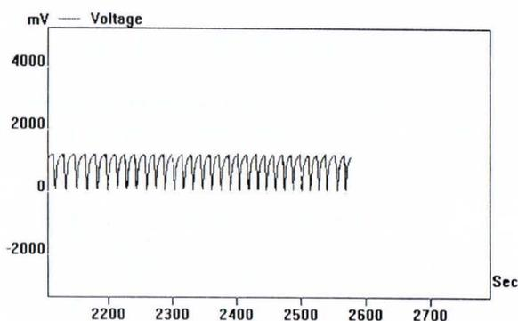
Figure 5. The charge-discharge cycles of ionic cell after 2600 sec.
