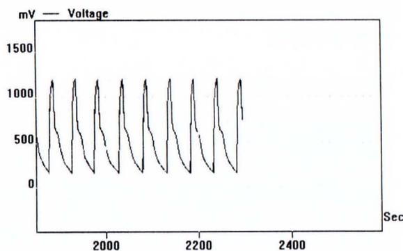
Figure 4. First charge-discharge result of ionic cell  $\text{Ag}/\text{AgI}-\text{AgPO}_3/\text{I}_2$
