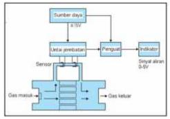
Gambar 6. Skema mass flow meter
