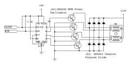
Gambar 5 Diagram Kendali Motor Stepper
