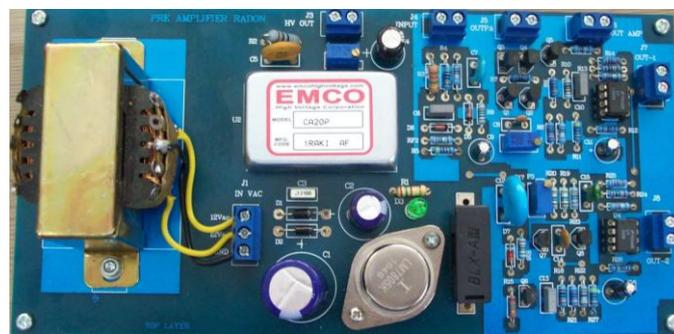
Gambar 7. Modul *pre amplifier* dan *high voltage*
