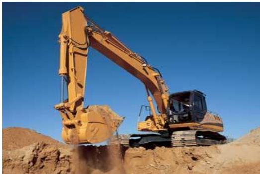
Gambar 6. Gambar Alat Excavator
