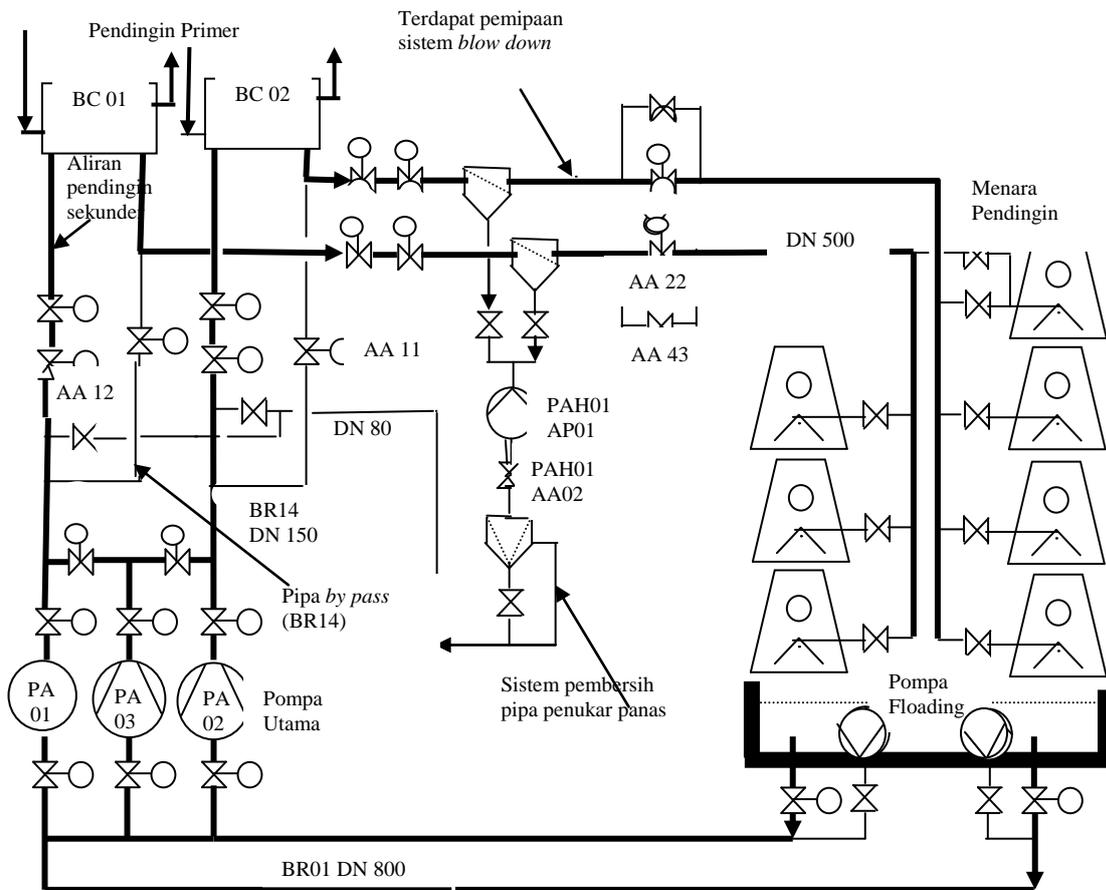
**Gambar 1.** Blok Diagram Sistem Pendingin Sekunder RSG-GAS.
