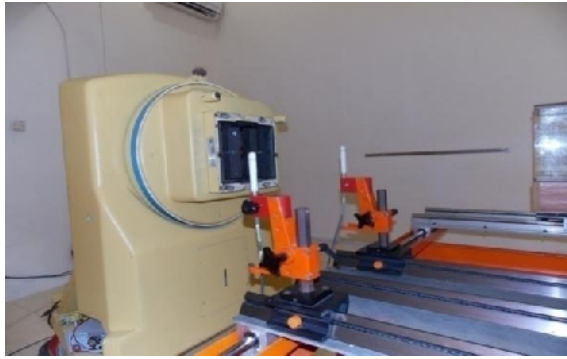
Figure 2. Two chambers used in this comparison. The transfer chamber on the right side and the reference standard chamber on the left side.
