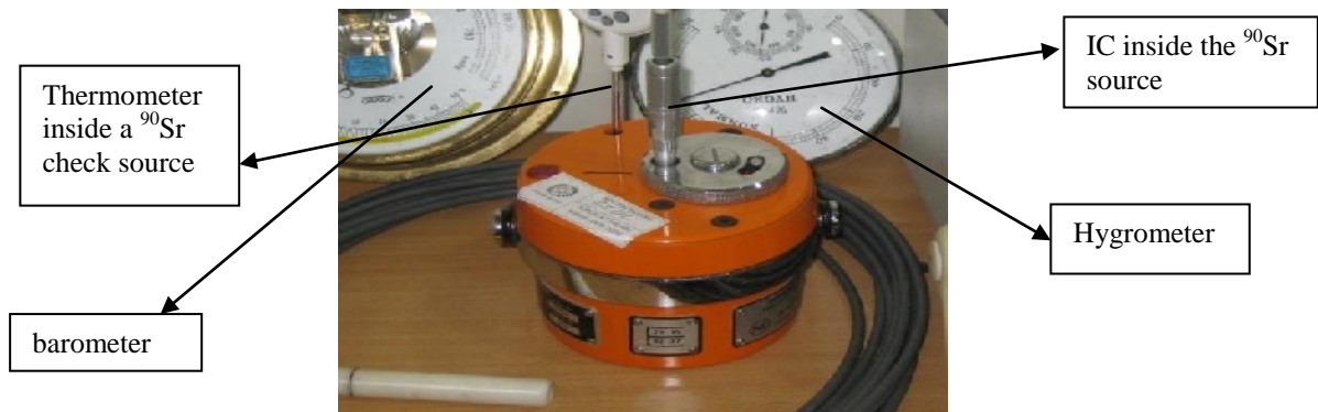
Figure 1. The set up of long term stability check of the chamber.
