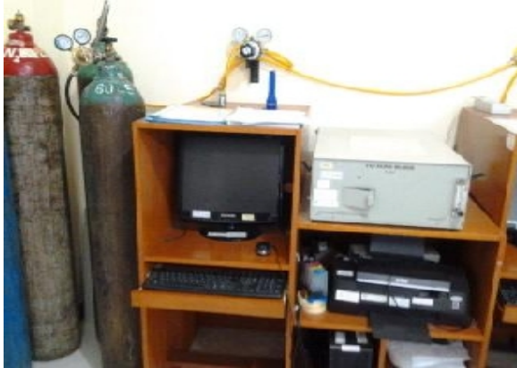
Figure 3. TLD Reader model TL 1010
