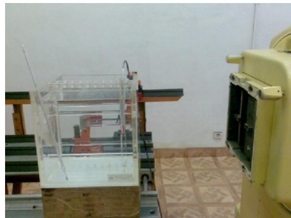
Figure 4. The setup for calibration of transfer chamber and the reference condition for the absorbed dose to water calibration coefficient (SSD 80 cm, FS 10 cm x 10 cm and 5 cm depth in water).
