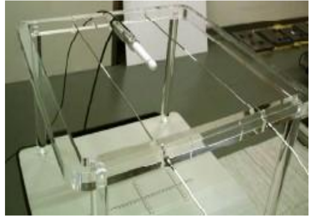
Figure 1. Special calibration jig for Nucletron mHDR machine.
