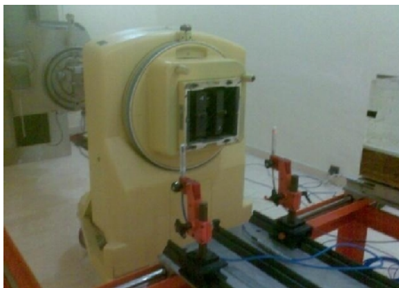
Figure 3. The setup for calibration of transfer chamber and the reference condition for the air kerma calibration coefficient (SCD 80 cm and FS 10 cm x 10 cm).
