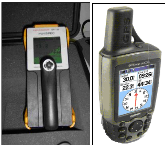
Figure 2. Surveymeter Exploranium GR130 portable (left) and GPS (Global Positioning System) Made by Garmin Model GPSMap 60CSx (right).
