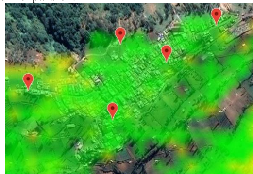
Figure 2. Five Nodes Coverage Area Simulation Result
