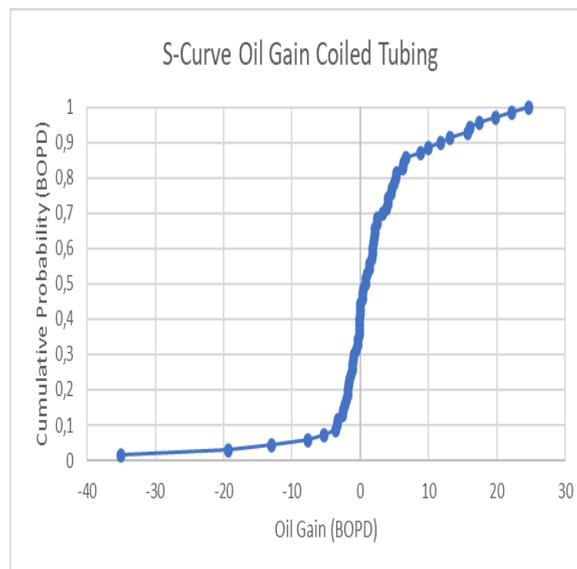
**Gambar 4.** Grafik S-Curve Oil Gain Menggunakan Metode Coiled Tubing
