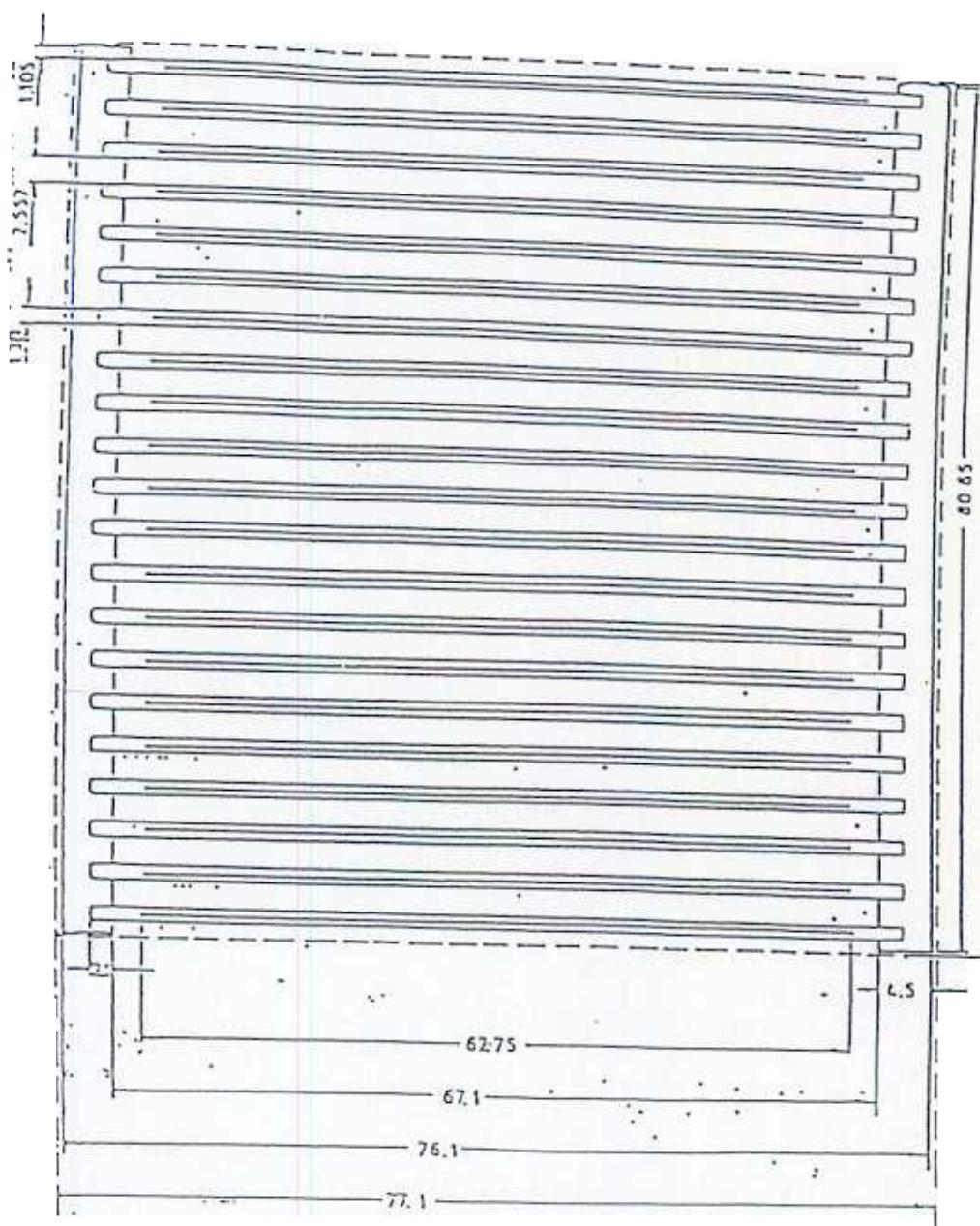
Gambar Horizontal Section Through Fuel Element
