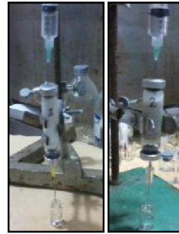
Gambar 4. Proses elusi kolom generator ^{188}\text{W}/^{188}\text{Re} berbasis MBZ
