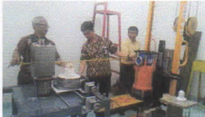
Gambar 1. Set-up percobaan Radioscopy, Sumber X-ray dan Sampel Stepwedge
