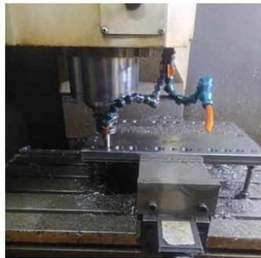
**Gambar 19. Proses Drilling**
