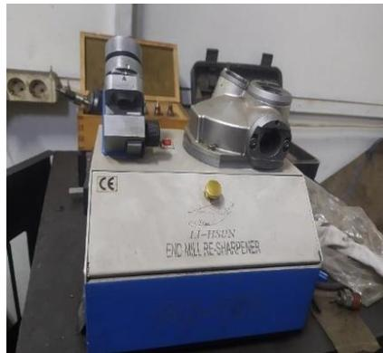
**Gambar 3.** *End Mill Sharpener*
