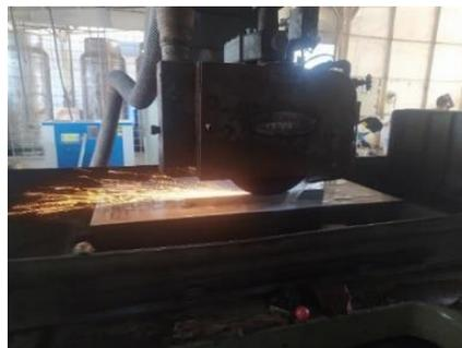
**Gambar 16.** Proses *Grinding*
