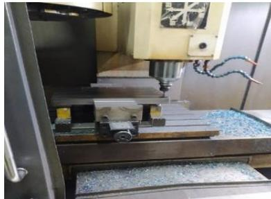
**Gambar 15.** Proses *Chamfering*
