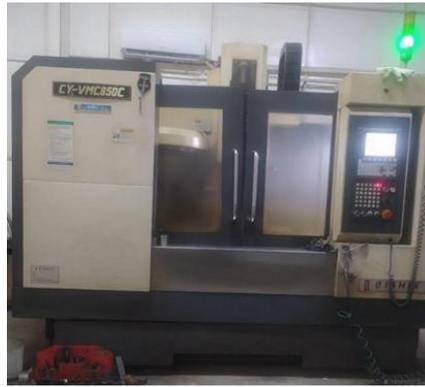
**Gambar 2.** Mesin CNC *Milling* Tipe CY-VM850C
