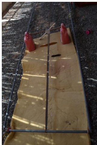
Figure 19. Siim tool (two pieces of woods sloped on two long steel tubes, stood on plastic cans) Photographed by Amal Al-Ismaili, North Sharqiyah, Oman, 2016.
