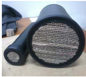
Figure 4 Samples of corrugated board mounted on an Impedance Tube
