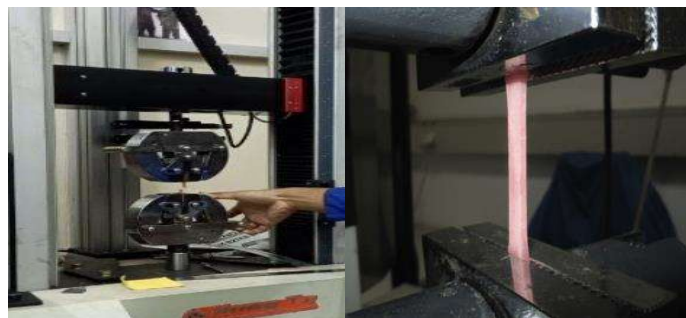
Figure 2. (A) Universal Testing Machine; (B) Specimen when pulled
