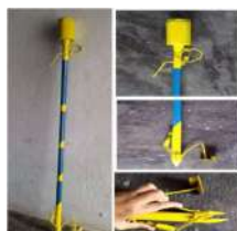
Gambar 2 Tugal double fungsi sistem pegas
