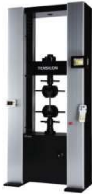
FIGURE 2. Universal testing machine tensilon RTF 2410.
