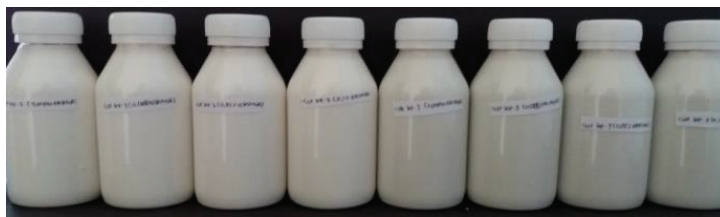
FIGURE 1. Anti-Aedes Aegypti Paint Formulation (Description of anti-mosquito paint from left to right; 2nd paint without extract (F5), 2nd paint with 0.025% extract (F6), 2nd paint with 0.05% extract (F7), 2nd paint with 0.1% extract (F8), 1st paint without extract (F1), 1st paint with 0.025% extract (F2), 1st paint with 0.05% extract (F3), 1st paint with 0.1% extract (F4)).
