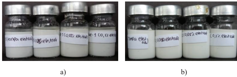
FIGURE 8. Organoleptic Test Result of Phase Separation Aspect a) First type (P-1) Paint on Second Week b) Second type (P-2) Paint on Second Week
