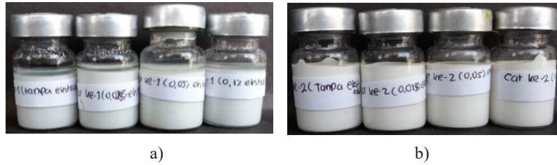
FIGURE 11. Organoleptic Test Result of Phase Separation Aspect a) First type (P-1) Paint on Fifth Week b) Second type (P-2) Paint on Fifth Week
