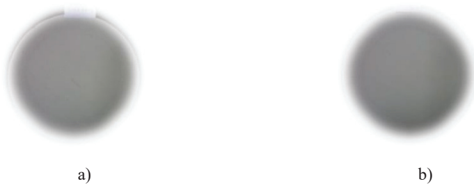
FIGURE 3. Alkali Resistance Test Results for a) First type (P-1) Paint with 0.05% ekstrak, b) First type (P-1) Paint with 0.1% Extract
