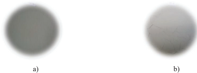
FIGURE 2. Alkali Resistance Test Results for a) First type (P-1) Paint without Extract, b) First type (P-1) Paint with 0.025% Extract
