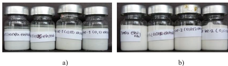
FIGURE 10. Organoleptic Test Result of Phase Separation Aspect a) First type (P-1) Paint on Fourth Week b) Second type (P-2) Paint on Fourth Week
