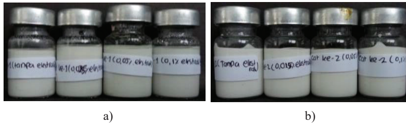
FIGURE 7. Organoleptic Test Result of Phase Separation Aspect a) First type (P-1) Paint on First Week b) Second type (P-2) Paint on First Week
