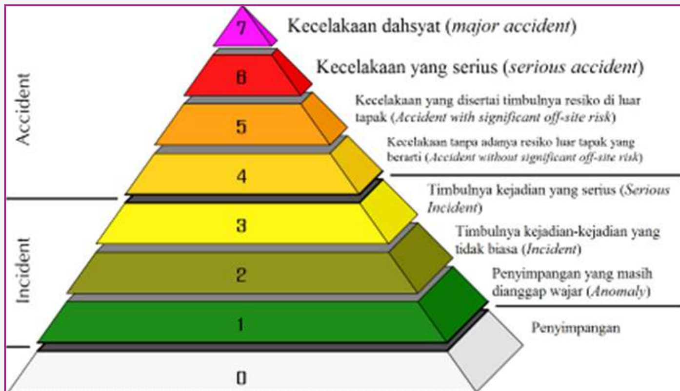
Gambar 5.3. Level Kecelakaan Nuklir (International Nuclear Event Scale / INES) Figure 5.3. International Nuclear Event Scale/ INES
