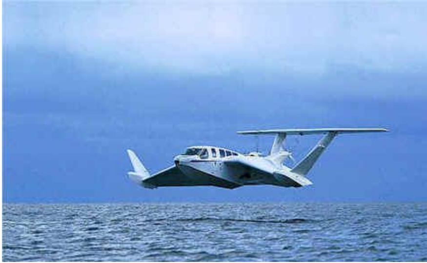
Gambar 1.1 Pesawat Flight Ship FS8 konfigurasi Lippisch ( https://sites.google.com/site/hoverwingwcraft ).
