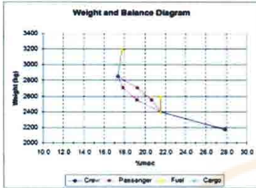
Gambar 8. Diagram Weight and Balance WISE-craft.
