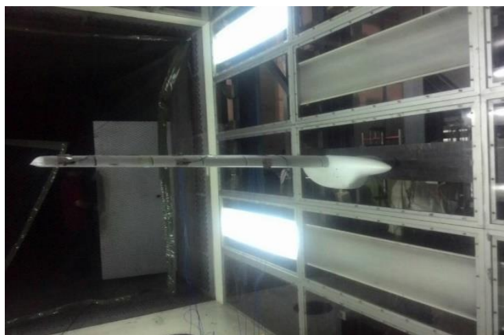
Figure 5 The half wing model installation in test section of wind tunnel.
