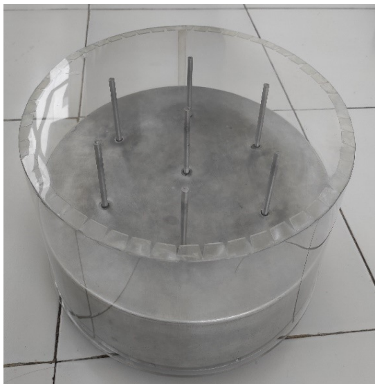
Fig. 6. The fabricated SPSA 915 MHz fully covered with the polycarbonate material.
