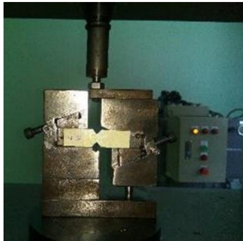
Figure 2. Setting for Shear Test.
