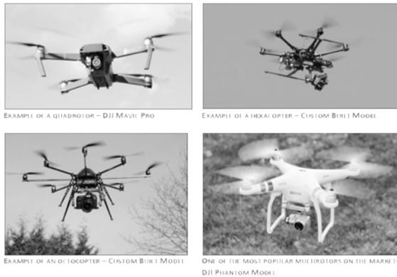
**Gambar 4.** Tipe-tipe Drone – Rotorcraft
