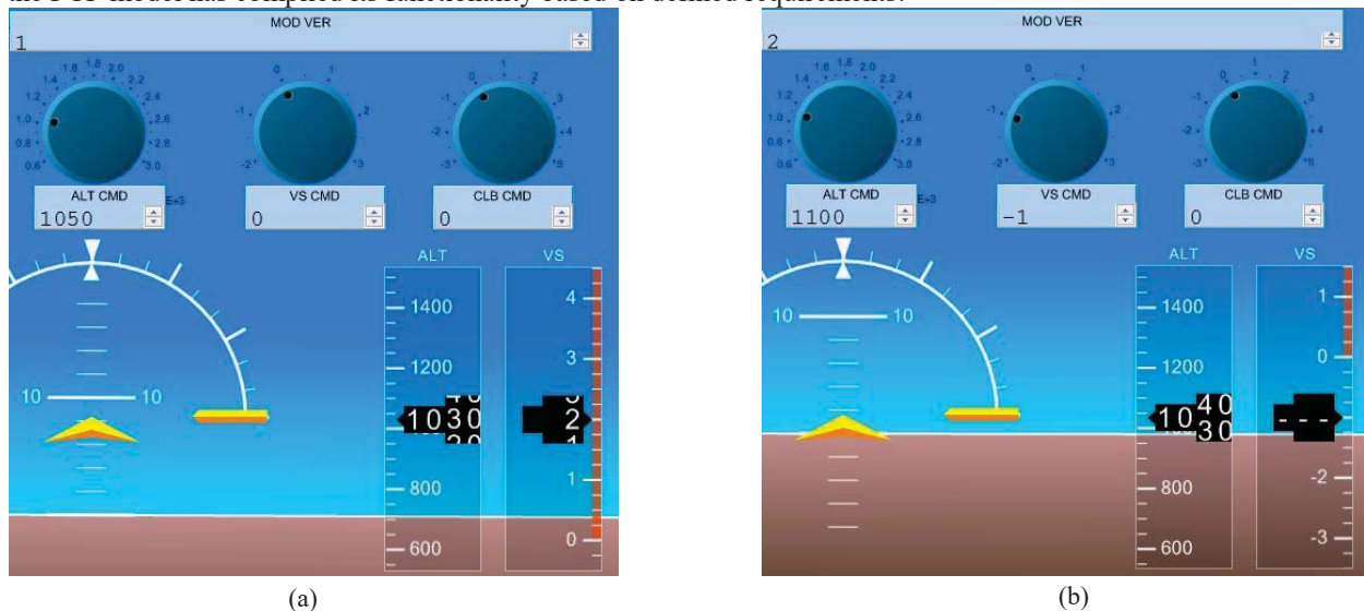
FIGURE 15. An example of vertical mode command and response in PFD design (a) vertical mode is set at 1 for altitude control, (b) vertical mode is set at 2 for vertical speed control.
