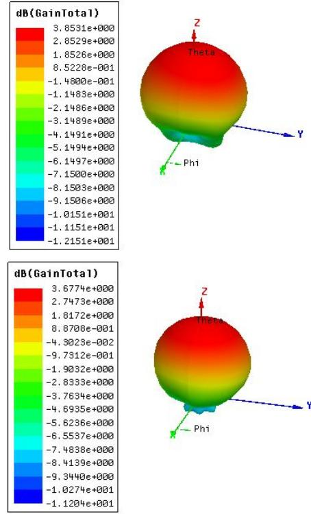
Fig. 6. Gain of Rectangular Patch & Truncated Corner
