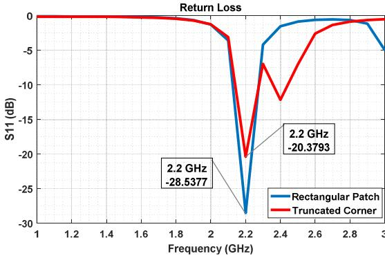
Fig. 4. Return Loss of Rectangular Patch & Truncated Corner
