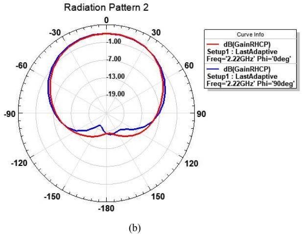
Fig. 9. (a) LHCP and (b) RHCP Gain of Antenna Truncated Corner
