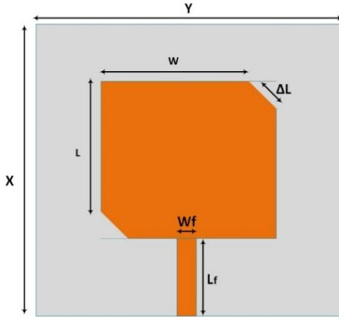
Fig. 3. Truncated Corner Microstrip Antenna Design
