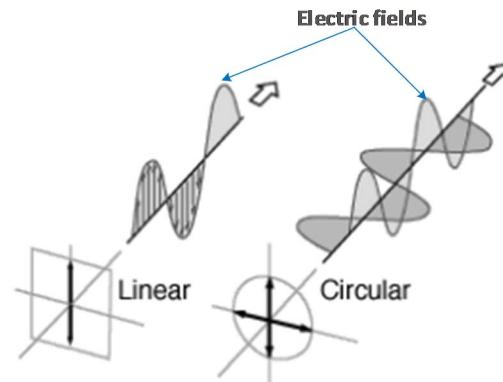
Fig. 1. Linear Polarization and Circular Polarization [10]
