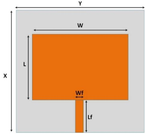
Fig. 2. Rectangular Patch Microstrip Antenna Design
