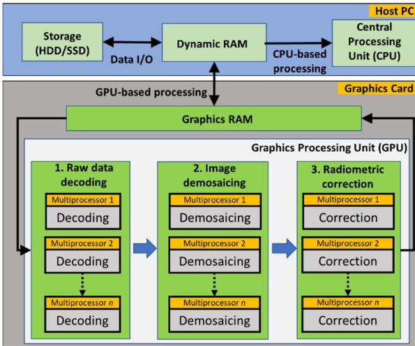
Fig 3. Block of proposed GPU-accelerated pre-processing for LAPAN-A2 imagery
