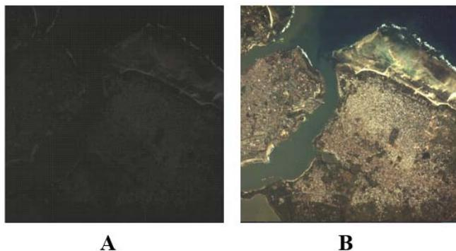
Fig 1. (A) Image of Mombasa taken from LAPAN-A2 SpaceCam and (B) is reconstructed RGB image using 'BGGR' array CFA filter.
