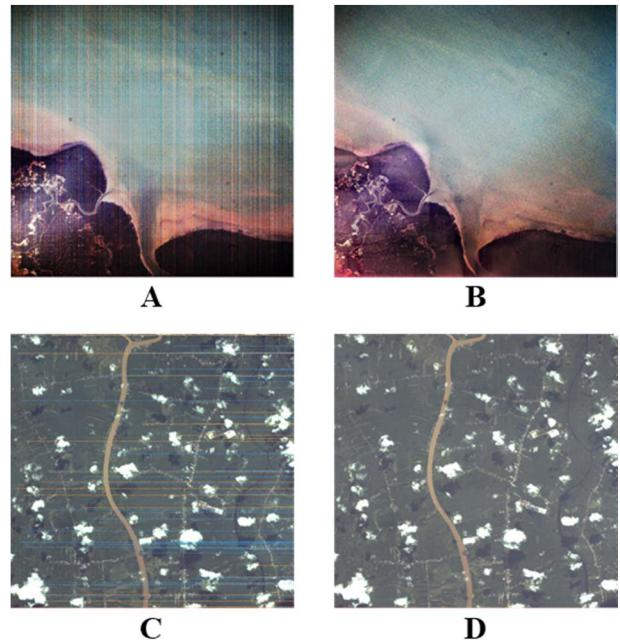
Fig 2. The results of image correction : (A) image disturbed by stripe noise; (B) result of stripe noise removal; (C) image disturbed by line-drop effect; and (D) result after applying line-drop correction [11], [12].
