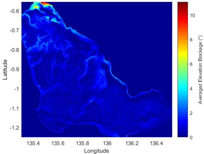
Fig. 8. Averaged elevation blockage map for a polar-orbiting satellite in Biak Island.
