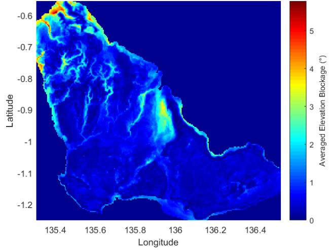
Fig. 7. Averaged elevation blockage map for an equatorial-orbiting satellite in Biak Island.
