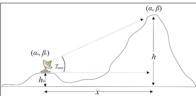
Fig. 2. Illustration of elevation blockage calculation.
