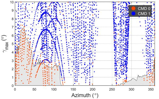
Fig. 4. Distribution of failed and successful commands of LAPAN-A2 and LAPAN-A3 satellites.
