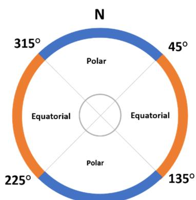
Fig. 6. Illustration of azimuth range for equatorial and polar-orbiting satellites.
