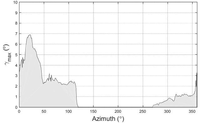
Fig. 3. Profile of maximum elevation blockage around the selected ground station.
