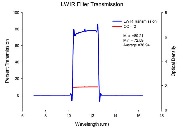
Fig. 12. LWIR Filter Transmission
