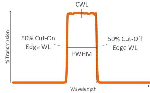
Fig. 6. Cut-on and cut-off wavelengths, center wavelength (CWL), and full-width at half-maximum (FWHM) for a bandpass filter.
