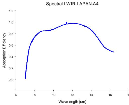
Fig. 4. Spectral Respons LWIR camera in LAPAN A4
