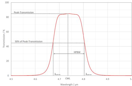
Fig. 5. Transmission range of a bandpass filter.
