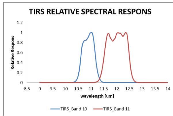
Fig. 2. Spectral Response TIRS bands 10 and 11 LANDSAT 8[7][8]
