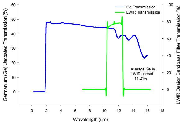
Fig. 13. LWIR Filter Vs Ge Uncoated Transmission
