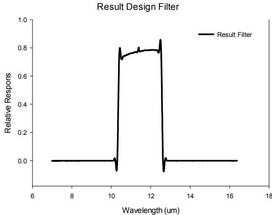
Fig. 10. LWIR Result Optical Bandpass Filter
