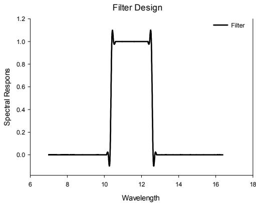
Fig. 9. LWIR Optical bandpass filter
