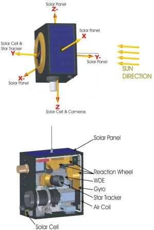
Fig. 1. Configuration of Lapan-Tubsat's attitude control system
