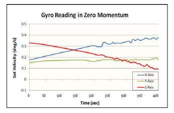
Fig. 3. Gyro Reading during Free Tumbling Condition
