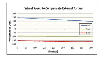
Fig. 4. Wheel Speed for External Torque Compensation
