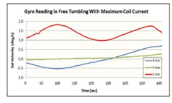
Fig. 5. Gyro Reading during Free Tumbling Condition with the Maximum Current Setting on Y Coil
