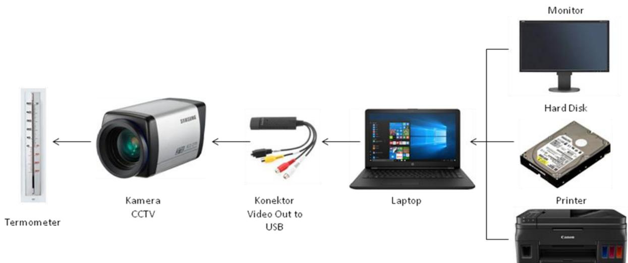
**Gambar 3. Alur monitoring skala termometer**
