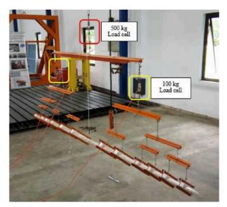
FIGURE 5. Load cell location on whiffletree
