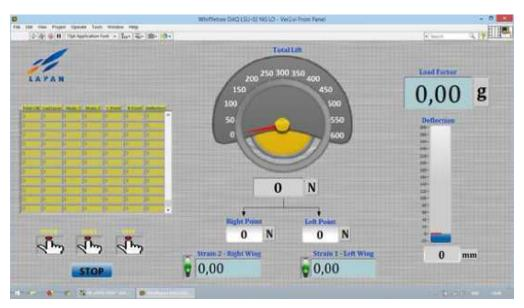
FIGURE 3. GUI design for wing static test
