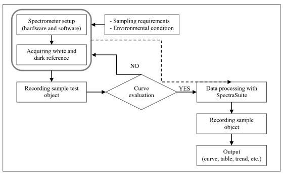
Figure 2. Scheme of acquiring data with spectrometer p. 25 (Kamal 2012)
