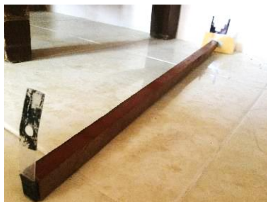
Figure 4. Bitterlich's stick with three BAF
