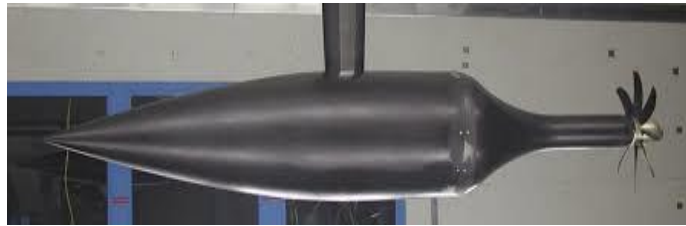
Fig. 2.4.2. Propeller mounted on an isolated nacelle
