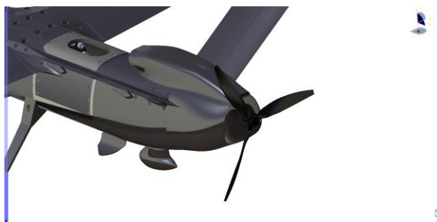
Fig. 2.4.3. Propeller mounted at original position on the model
