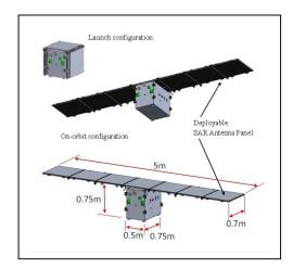
Fig. 2.1. Overview of small satellite with X-band SAR
