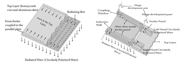
Fig.2.2. (a) Antenna panel from feeder side.
