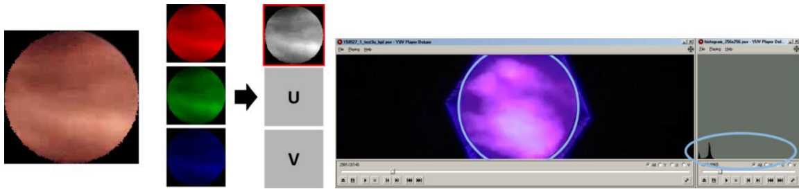
Fig. 2.2. a) Extraction of brightness and luminosity estimation from captured image b) Screen capture of image processing software
