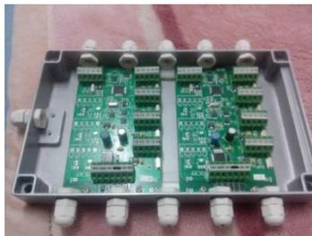
Gambar 3-1 PCB Indikator Load Cell 10 Kanal
