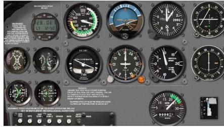
Gambar 2-1. Panel instrumen Cessna 172 S[5]
