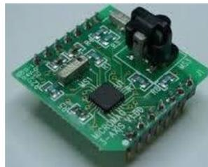
Gambar 2-3 Sensor Magnetometer
