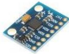
Gambar 2-2 Sensor Gyroscope
