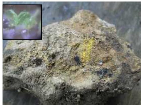
Figure 2: Gummite (yellow) and autunite (inset, 100x magnification) as radioactive minerals in leucitic basalt rock.
