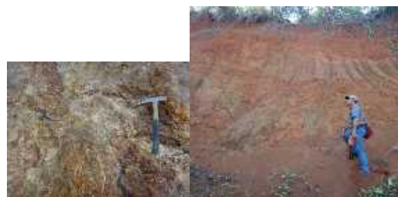
Figure 3: Altered leucite basalt rock (left) and lateritic soil (right) containing high concentration of thorium.
