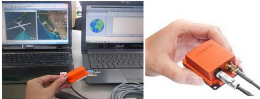
Figure4.Theinertial sensor being used to measure attitude of the flying vehicle.
