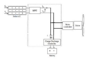
Fig. 2.Electric control system of a solar-powered LSU-01
