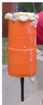
Fig. 1. Realization of the meteorological payload. (a) Payload bottom view. The temperature and relative humidity sensor pipeline was shown by red cross. The pressure sensor (black) was connected to transparent pipe. (b) Payload top view after it was placed into PVC pipe. (c) Payload side view after it has just casted using polyurethane. (d) Ready to launch payload.
