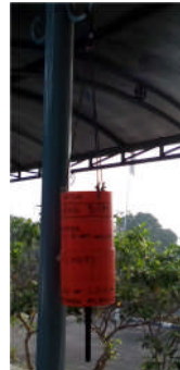
Fig. 1. Realization of the meteorological payload. (a) Payload bottom view. The temperature and relative humidity sensor pipeline was shown by red cross. The pressure sensor (black) was connected to transparent pipe. (b) Payload top view after it was placed into PVC pipe. (c) Payload side view after it has just casted using polyurethane. (d) Ready to launch payload.
