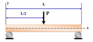
Fig. 2. Three point bending test
