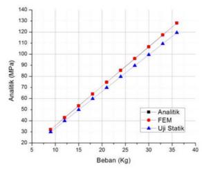
Fig. 14. Comparison of analytical, numerical(FEM), and experiment test
