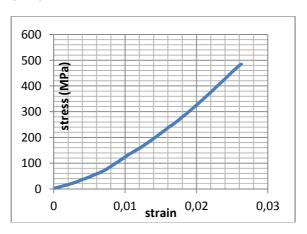
Fig. 1. Relationship stress - strain on tensile testing of e-glass composite UD  $0^0$
