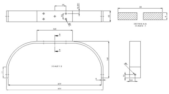
Fig. 5. Main Landing Gear Structure Dimension of LSU-02-02
