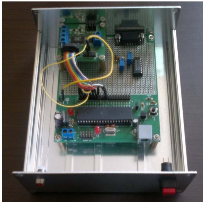
Gambar 1.2. Prototipe multi frekuensi signal beacon.
